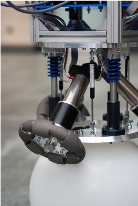
*Figure 5 Drive System: Motor EC-4pole 30, Planetary Gearhead GP 42 C, Angular Encoder HEDL 5540, Omniwheel*
